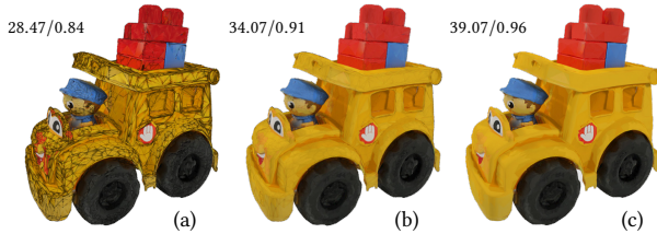
Figure 11: We compared the interpolation-based scheme (a) and the differentiable-rendering-based scheme (b). The texture quality is further improved by our normal-based camera pose sampler (c). The annotated numbers above each example are in the format of PSNR/MS-SSIM.
