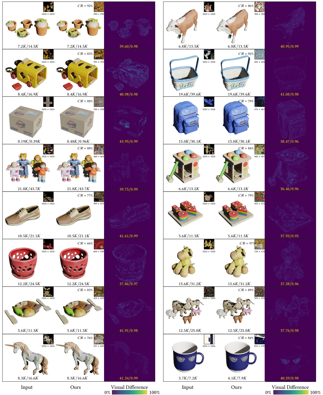
Figure 15: For each model, we provide information on the number of vertices and faces of the mesh, as well as the resolution of the texture, for both the input and the result. Additionally, we report the compression rate of the texture CR and the visual appearance preservation quality in terms of PSNR/MS-SSIM.
