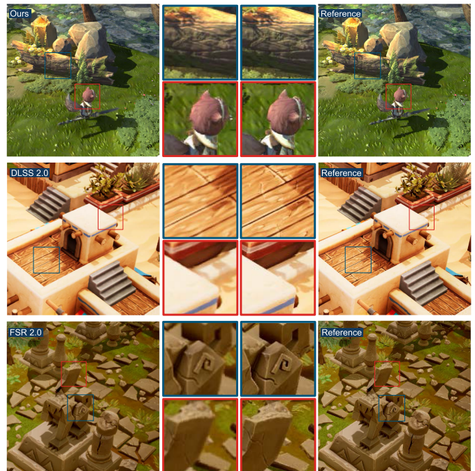
Fig. 9. Visual comparisons of our method, DLSS 2.0 [7], and FSR 2.0 [24] for scale factor \times 2 . The images in blue boxes compare different texture reconstruction methods, whereas the images in red boxes compare reconstructions on disoccluded regions.
